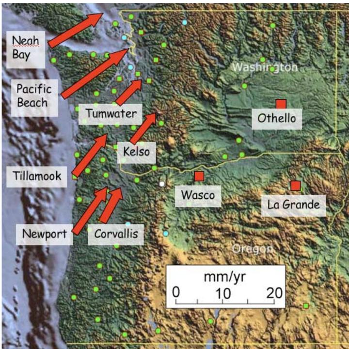
**LEFT:** Image from PowerPoint presentation shows all the motion vectors plotted on a map of Oregon and Washington. Notice that all the stations are moving in a northeasterly direction because this is the direction that the Juan de Fuca Plate is moving with respect to the North American Plate. The Coast Range is there because the land is deforming and rising in response to the forces pushing on it by the subducting Juan de Fuca Plate.
