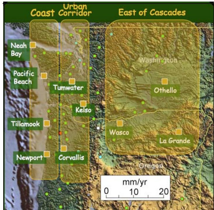
Map of 10 Plate Boundary Observatory GPS stations. The yellow blocks show the three regions reflecting GPS motion at different distances from the plate boundary. Coastal stations are being pushed towards the northeast faster than are the stations in the urban corridor and the stations east of the Cascades are basically not moving
