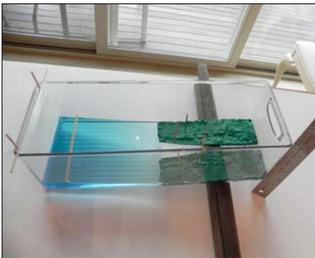
**Figure 4:** Side view of the wave tank.
